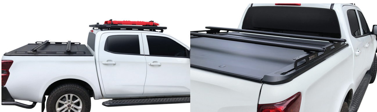
Ute fit - Spine fitted into track with TRIM HD bars
