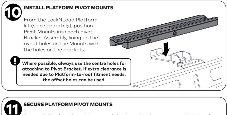
Secure all Platform Pivot Mounts with 2x 16 mm M6 Capscrews with Washer from LockNLoad Platform kit as shown.
