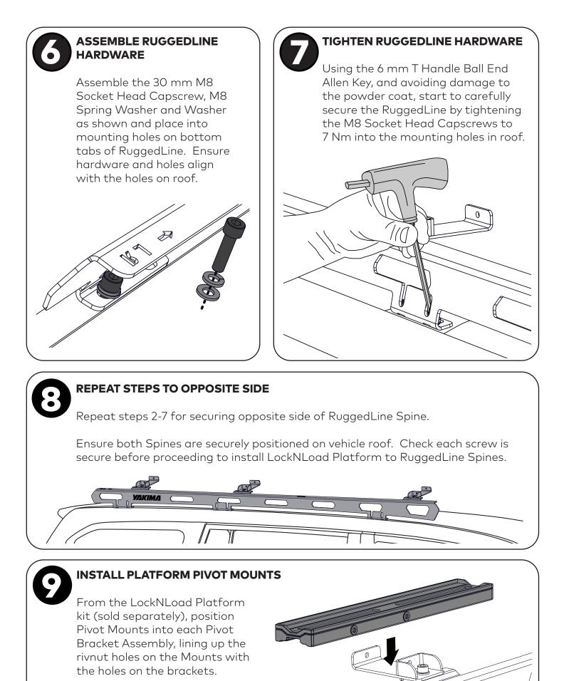
Where possible, always use the centre holes for attaching to Pivot Bracket. If extra clearance is needed due to Platform-to-roof fitment needs, the offset holes can be used.
