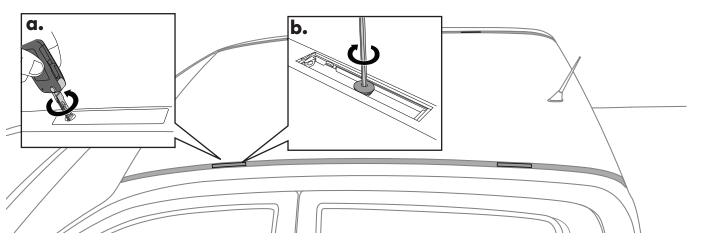
Remove all four mounting plugs using the provided 5 mm T Handle Ball End Allen Key.
