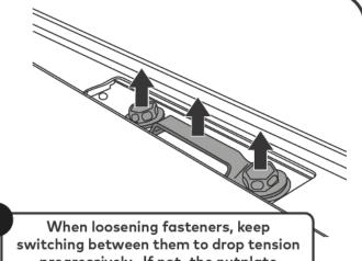
progressively. If not, the nutplate inside the roof cavity may come loose.
