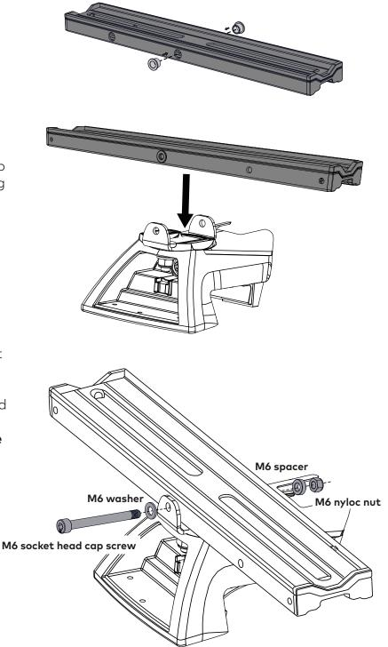
**NOTE -** The pivot mount assembly will still have movement after securing which is intended.
