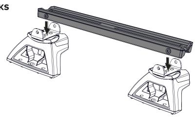
**NOTE -** The Mounting Block assembly will still have movement after securing which is intended.
