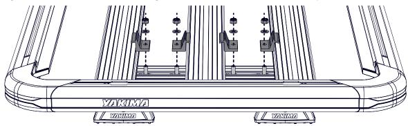
NOTE - Do not to over tighten Slat Clamps past 7 Nm as this may reduce clamping force.
