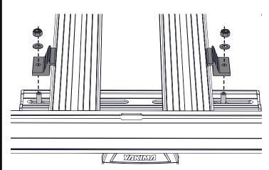
NOTE - Do not to over tighten Slat Clamps past 7 Nm as this may reduce clamping force.
