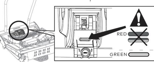
NOTE - Ensure the lock is in the unlock position and the indicator window is completely green.
