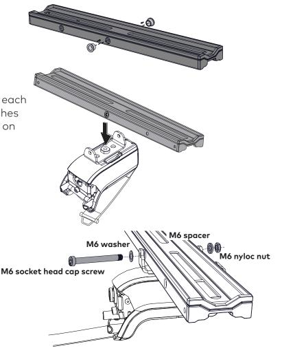
**NOTE -** The pivot mount assembly will still have movement after securing which is intended.
