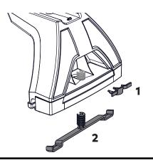
LOOSEN GUTTER MOUNT PLATE
