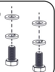
Loosely finger tighten Nut Plates to Legs as shown using the screw assemblies from the previous step.
