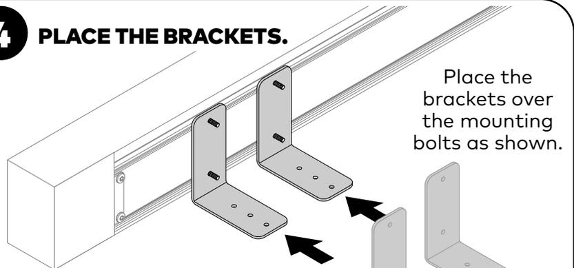
Place the brackets over the mounting bolts as shown.
