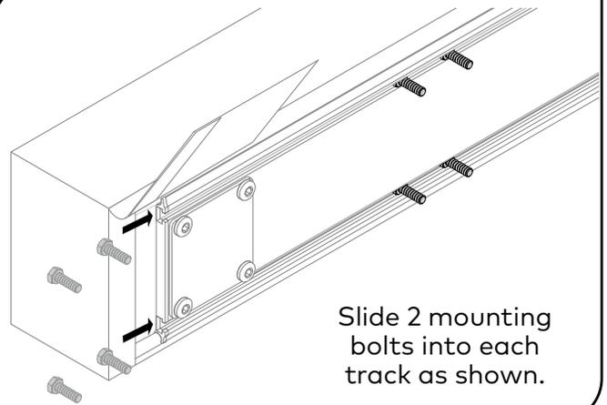
Slide 2 mounting bolts into each track as shown.
