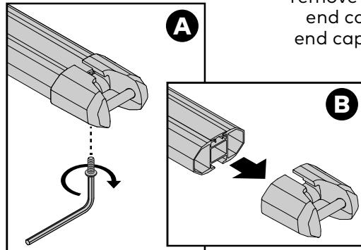
Use the hex wrench to remove the screw under the end cap and remove one end cap from each HD Bar.
