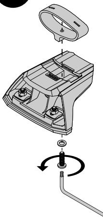
Place the metal crossbar adapter that came with your CoreBar. Use the T30 wrench to loosely attach the adapter using an M6 screw and washer as shown.
