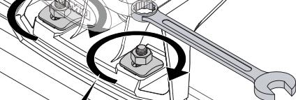
**NOTE:** Periodically check that the hardware is tight. Retighten to 4 Nm as necessary.
