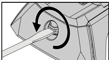
Use a flat-head screwdriver, or a coin, to unlock the covers and remove them.
