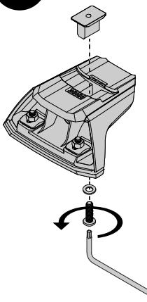
Place the metal crossbar adapter that came with your adapter kit. Use the T30 wrench to loosely attach the adapter using an M6 screw and washer as shown.
