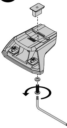
Place the metal crossbar adapter that came with your adapter kit. Use the T30 wrench to loosely attach the adapter using an M6 screw and washer as shown.
