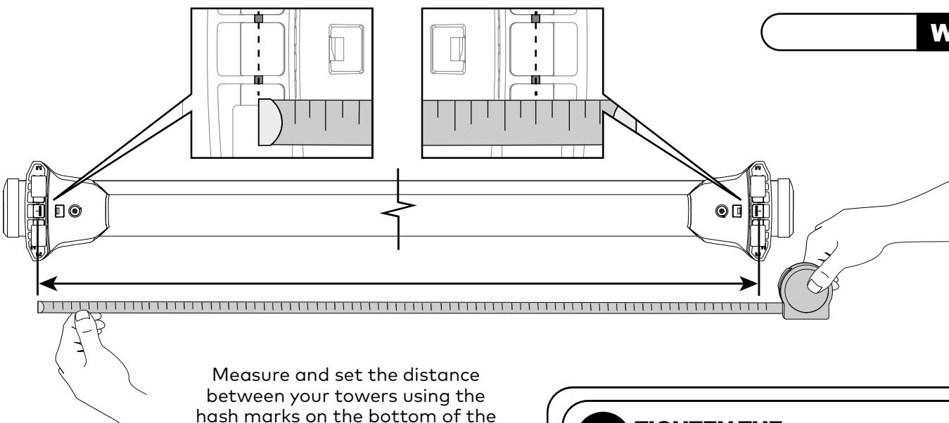
Measure and set the distance between your towers using the hash marks on the bottom of the towers as shown. Set the distance between the hash marks to the W2 measurement you recorded in step 1. Center the bar so there is equal overhang on each side.
