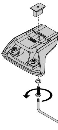
Place the metal crossbar adapter that came with your JetStream Bar. Use the T30 wrench to loosely attach the adapter using an M6 screw and washer as shown.
