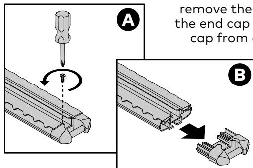
Use a Philips screwdriver to remove the screw at the top of the end cap and remove one end cap from each Trim HD Bar.
