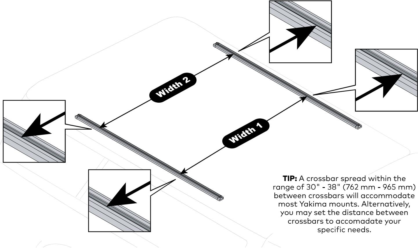
**TIP:** A crossbar spread within the range of 30" - 38" (762 mm - 965 mm) between crossbars will accommodate most Yakima mounts. Alternatively, you may set the distance between crossbars to accommodate your specific needs.
